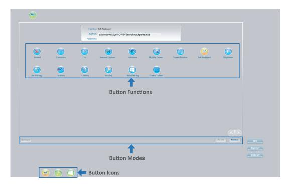
The Button Icons are located close to physical button locations. The icons show current assigned function. Button functions section will list all available functions for current system model.
